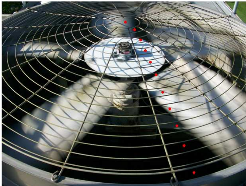
Figure 2 - Fan with measured locations marked in red
